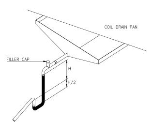
Dim 'H' = total static pressure mm Wg + 25mm minimum
