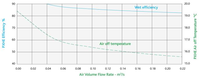
CF350 Heat exchanger performance at 20°C (50% RH) return air and -5oC (100% RH) fresh air. Approx. 16.2°C air off at 0.128m3/s.
