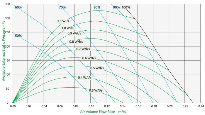
Curves represent performance of a unit with integral LPHW coil and F7 filter in mean condition. Tolerance: +/-5%. SFP values shown are for one fan.
