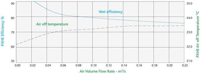
CF350 Heat exchanger performance at 22°C (50% RH) return air and 28°C (50% RH) fresh air. Approx. 23.3°C air off at 0.128m³/s.
